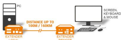
POINT TO POINT CONNECTION
