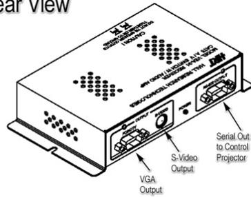
As seen in the above diagrams, the connection between the receiver and the projector could be comprised of VGA, S-Video, and RS232. These cables are not supplied and must be purchased separately.
